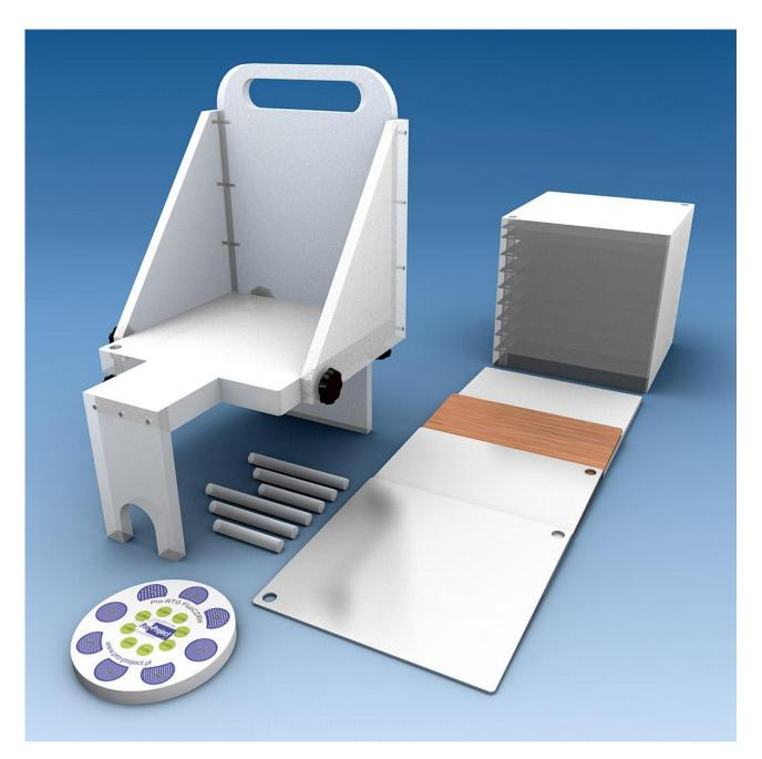
Compact and easy to use phantom for performance evaluation of fluoroscopic systems according to Center for Devices and Radiological Health (CDRH) specifications. It also meets recommendations of AAPM Report No. 60 "Instrumentation Requirements of Diagnostic Radiological Physics". It is optimized for both underand over-table fluoroscopic tubes.
